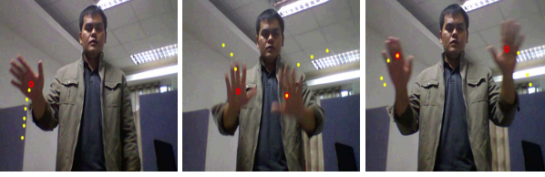
Fig. 4. the trajectory of hand tracking with Condensation Algorithms
