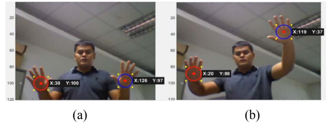
Fig. 3. Hand localization is (a) Hand localization with a circle and centroid point (b) Search area around the detected hands.
