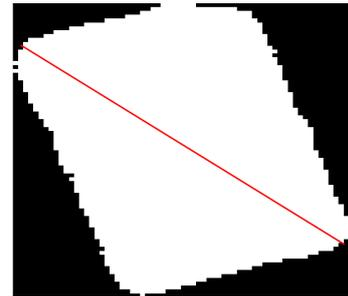
Fig. 4 Drawing Feret diameter in red line in case of size 4 mm which obtain from library
