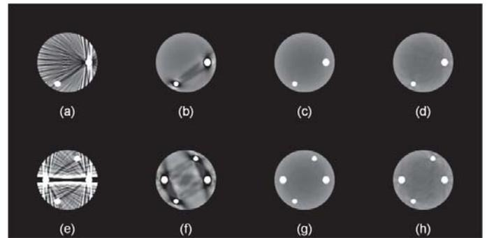
Figure 2. (a & e) Uncorrected, (b & f) standard MAR, (c & g) IMAR-TVM, and (d & h) proposed IMAR-PDART images of Phantom 1 and Phantom 2 are provided in the 1st and 2nd rows, respectively.
