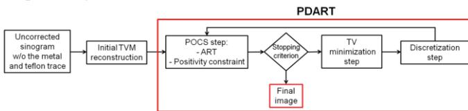
Fig. 1 Flow diagram of the proposed PDART scheme. PDART process was implemented after an initial number of conventional TVM iterations. This was followed by a sequence of POCS, TV, and discretization steps until a prior image was reconstructed after 5 PDART iterations.
