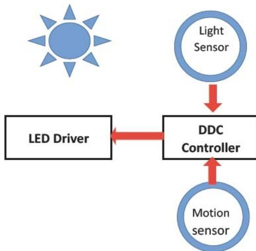
Fig. 5 Lighting control (Original Scheme)
