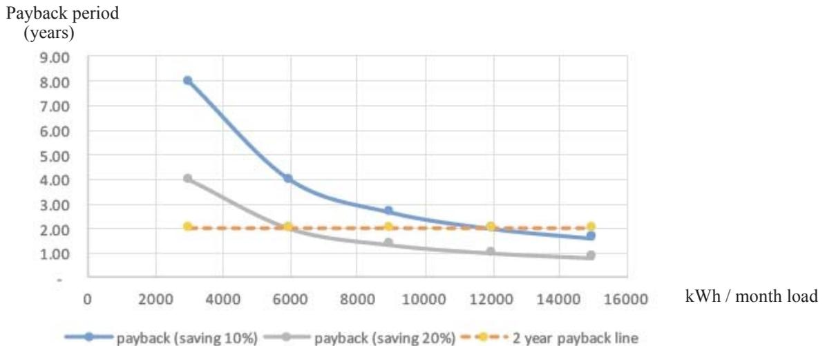
Fig. 8 Payback period vs. kWh per month load
