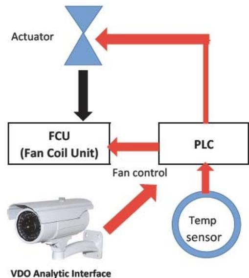
Fig. 6 Air-conditioning control (Proposed Scheme)
