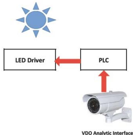
Fig. 7 Lighting control (Proposed Scheme)
