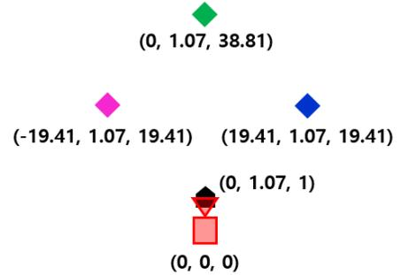
Fig. 5. Relative position of the bases and the virtual camera.
