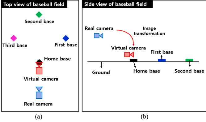
Fig. 2. Proposed method system. (a) A top view image of the system. (b) A side view image of the system.
