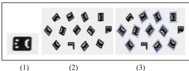
Fig. 2. (1) Pattern Image (2) Input Image (3) Result of multi-angle matching
