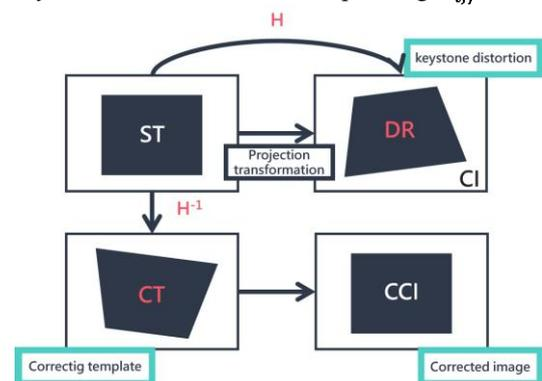
Fig. 1. Projection distortion and correcton
