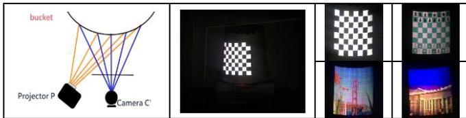
Fig. 9. Correction for curved bucket projection
