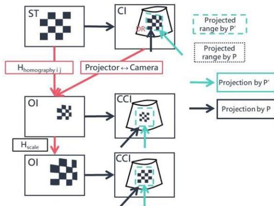
Fig. 6. Obtaining correction template for curved projection surface
