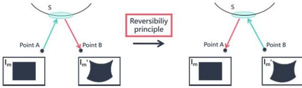
Fig. 2. Reversing projection direction resulting images unchanged
