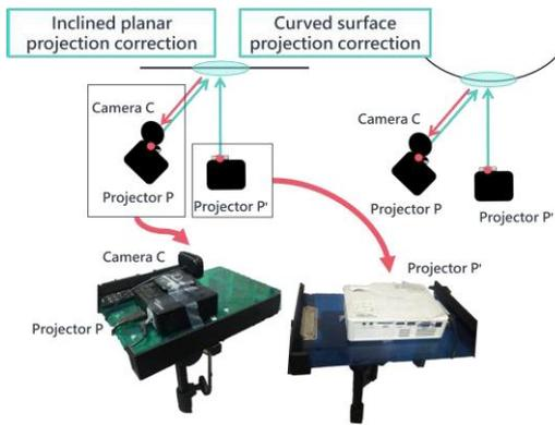
Fig. 5. Stacking projector and replacing camera together
