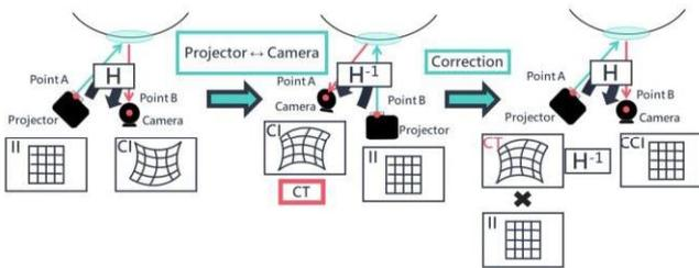
Fig. 3. Application of projection reversibility principle
