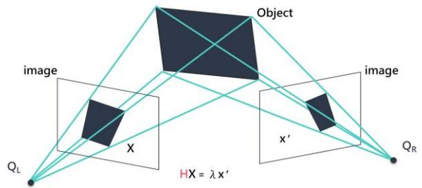
Fig. 4. Epipolar geometry
