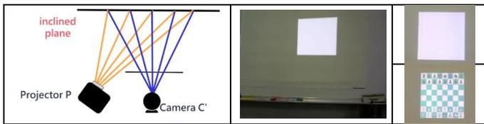
Fig. 8. Correction for Inclined plane projection
