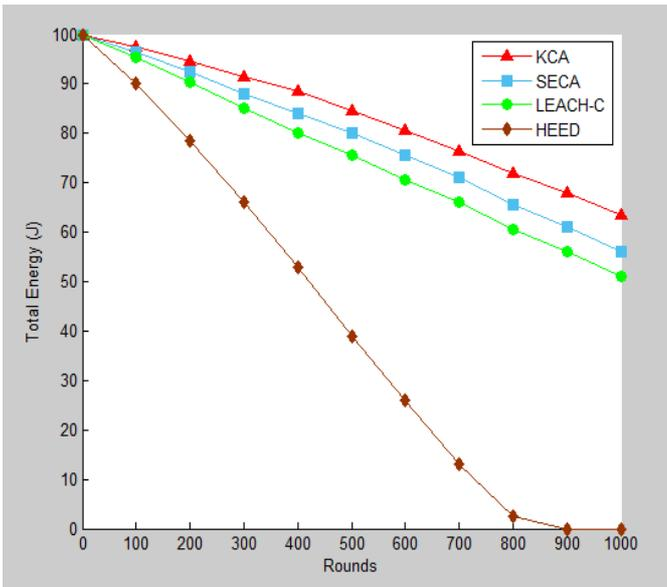
Fig. 2. Residual energy comparison
