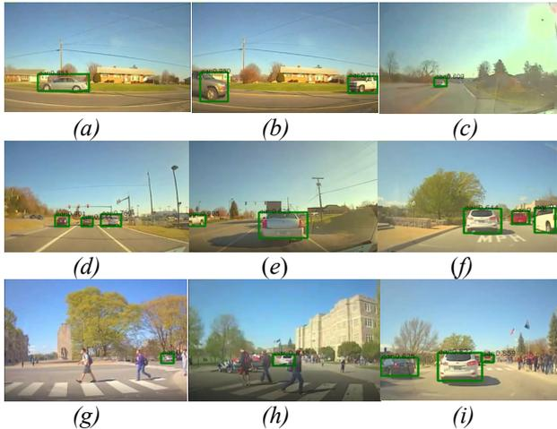
**Figure 5. Vehicle detected in the videos from SHRP 2 NDS database.**
