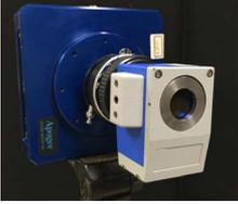
Fig. 2. 16bit CCD camera and NIR tunable filter
