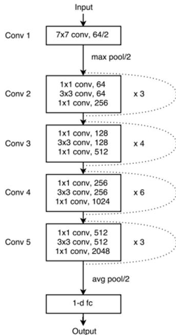
Fig 2. Structure of deep residual age estimation model
