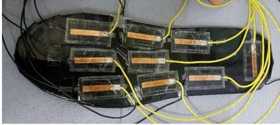
Fig. 1 The force sensor for foot pressure measuring
