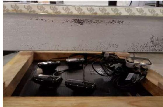
Fig. 3 four digital cameras underneath the platform
