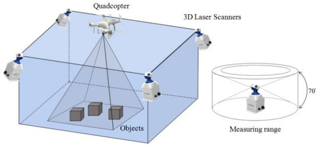
Fig. 1. Configuration of prototype system.
