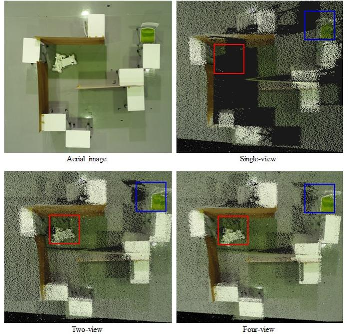
Fig. 4. Full color 3D point clouds from bird's-eye view.
