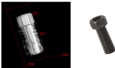
**Fig. 7. Reconstruction Screw**
