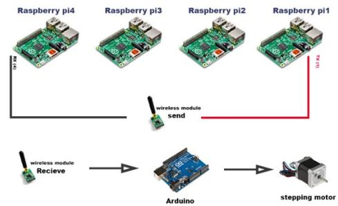
**Fig. 3. A schematic of the system**
