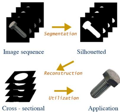
**Fig. 1. The process diagram of the photographic tomography**
