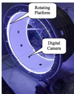
**Fig. 2. Acquisition system of embedded photographic tomography**
