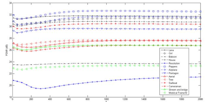
Fig. 7. The impact of the Leclerc constant (T) on the PSNR performance of the proposed SI-SR under the noisy at SNR=35 dB status
