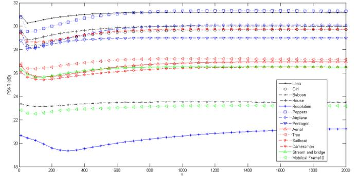
Fig. 6. The impact of the Leclerc constant (T) on the PSNR performance of the proposed SI-SR under the noisy at SNR=30 dB status
