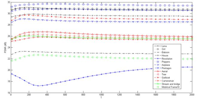
Fig. 8. The impact of the Leclerc constant (T) on the PSNR performance of the proposed SI-SR under the blurring status
