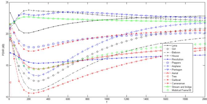
Fig. 3. The impact of the Leclerc constant (T) on the PSNR performance of the proposed SI-SR under the noisy at SNR=15 dB status
