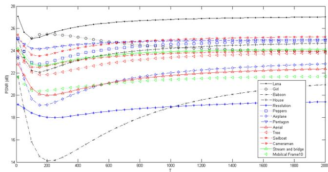
Fig. 4. The impact of the Leclerc constant (T) on the PSNR performance of the proposed SI-SR under the noisy at SNR=20 dB status
