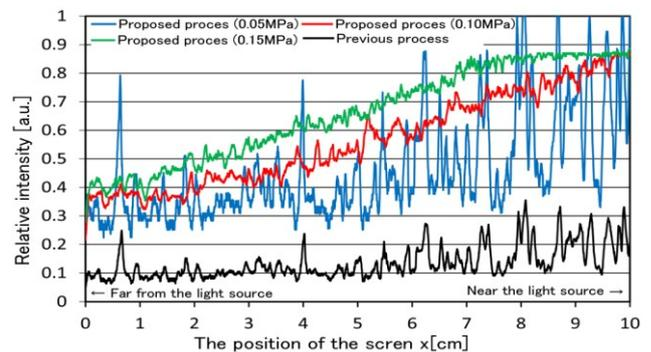
Fig.8 Change of the relative light intensity on the screen with respect to the position.
