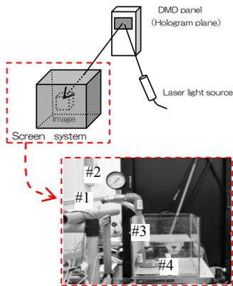
Fig.1 Optical setup for reconstruction of 3D holographic images in the projected process
