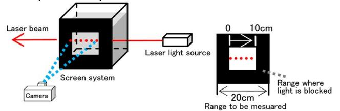
Fig.6 Measurement of the distribution on the light intensity on the screen
