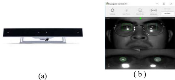
Figure 9. (a) Gazepoint GP3 Eye tracker module (b) Eye tracking by Gazepoint GP3 Eye tracker.
