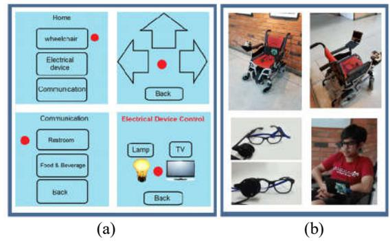
Figure 4 (a) Cursor control on the Raspberry Pi Screen (b) wheelchair-controlled
