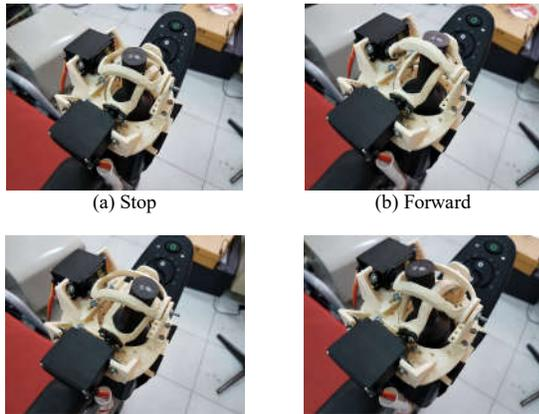
Figure 6 the wheelchair-controlled module (2 dimensional rotating stage)
