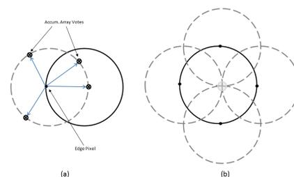
Figure 1 Circle Hough transform Algorithm [3]
