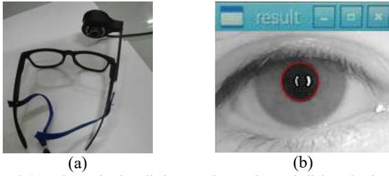
Figure 2 (a) webcam that installed on eyeglass as (b) eye ball detection based on circle Hough transform
