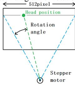
Fig. 14. Calculation of rotation angle
