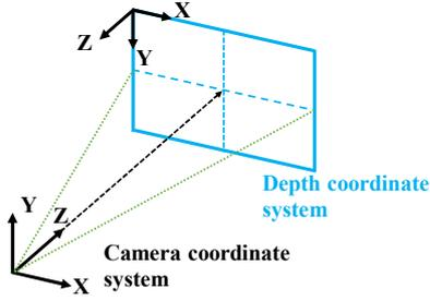
Fig. 9. A pattern diagram of conversion of the coordinate system
