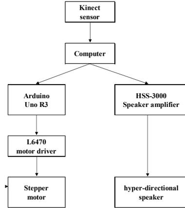
Fig. 11. Connecting devices
