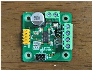
Fig. 4. Motor driver (L6470<sup>[9]</sup>)
