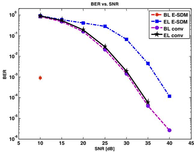
Figure 4. BER of the base and enhancement layers vs. SNR.
