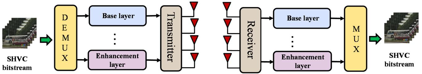
Figure 3. Proposed video transmission scheme for SHVC bitstreams with the MIMO E-SDM system.
